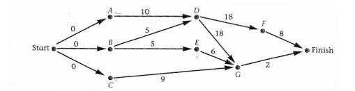
7. Determine the minimum project time and the critical path for the following graph.
